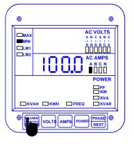
Step 2: a. Press *MAX/MIN/LIMITS* twice to access the min value for Amps A.
