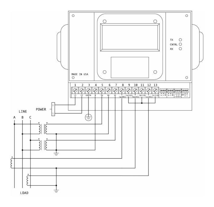
II. Three-Phase, Three-Wire Open Delta with two CTs and two PTs. Special Programming Required.
