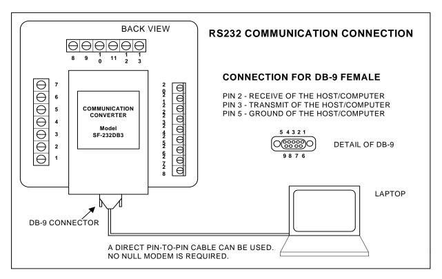
Figure 4.1: RS232C Communication Connection Installation
