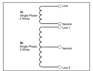
Figure 1.1: Single Phase System: (A) Two-Wire, (B) Three-Wire
