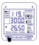
Step 1: a. Press MAX/MIN/LIMITS once to access max value; twice to access min value.
