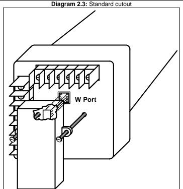
Diagram 2.4: Optional Communication Converter or DC Output Module Installation \* Recommended wire gauge is 20 AWG for DC Output or RS485 options.
