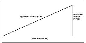
Figure 1.2: Relationship between apparent, real and reactive power
