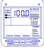
Step 1: a. Press and hold down PHASE/NEXT. While holding down PHASE/NEXT, press AMPS to access the display.
