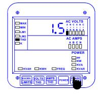
**Step 2:** Press and hold the **POWER** button to scroll through the instantaneous single-phase power readings.
