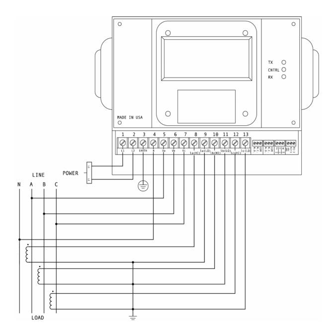
IV. Three-Phase, Four-Wire System Wye with Direct Voltage and CTs.
