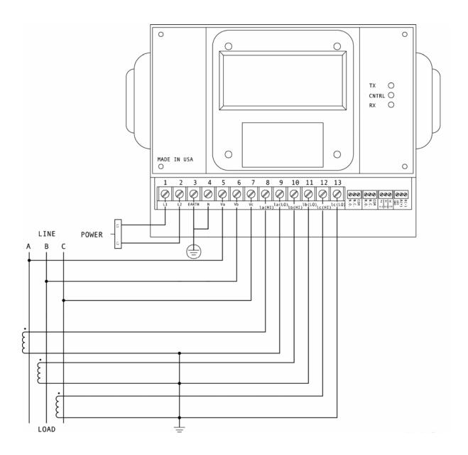
I. Three Phase, Three-Wire System Delta with Direct Voltage and CTs.
