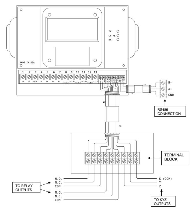
**Figure A-3.1:** Wiring Diagram of DMMS 300B RS485 Communication and Relay Output Installation.
