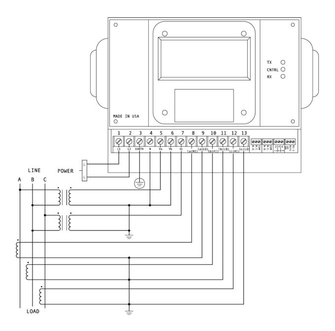
III. Three-Phase, Three-Wire Open Delta with three CTs and two PTs. Special Programming required.
